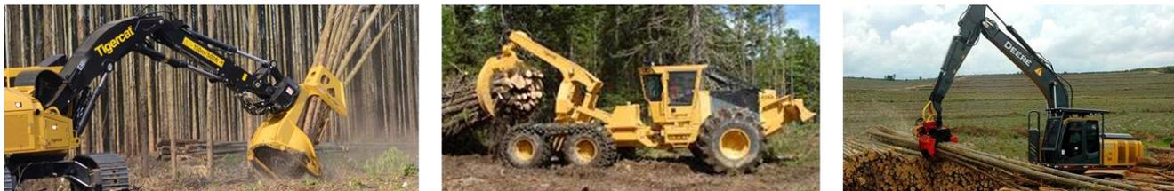
**Figura 10. Sistema *cut to length*: *harvester* e *forwarder***
